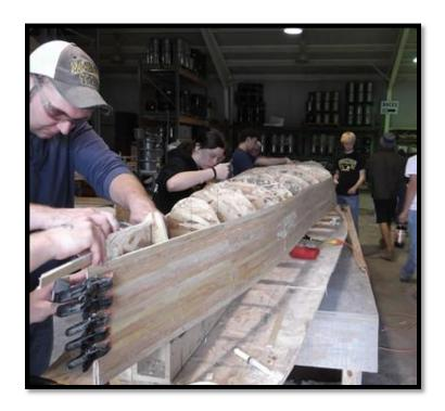
Before approving Genoa's hull design the team built a prototype canoe, Laker, to test the new design. Laker proved that the design would satisfy its goals and set a new standard for the team's future prototype canoes after being built within a week out of luann plywood strips at a third the cost of a traditional cedar strip canoe.
