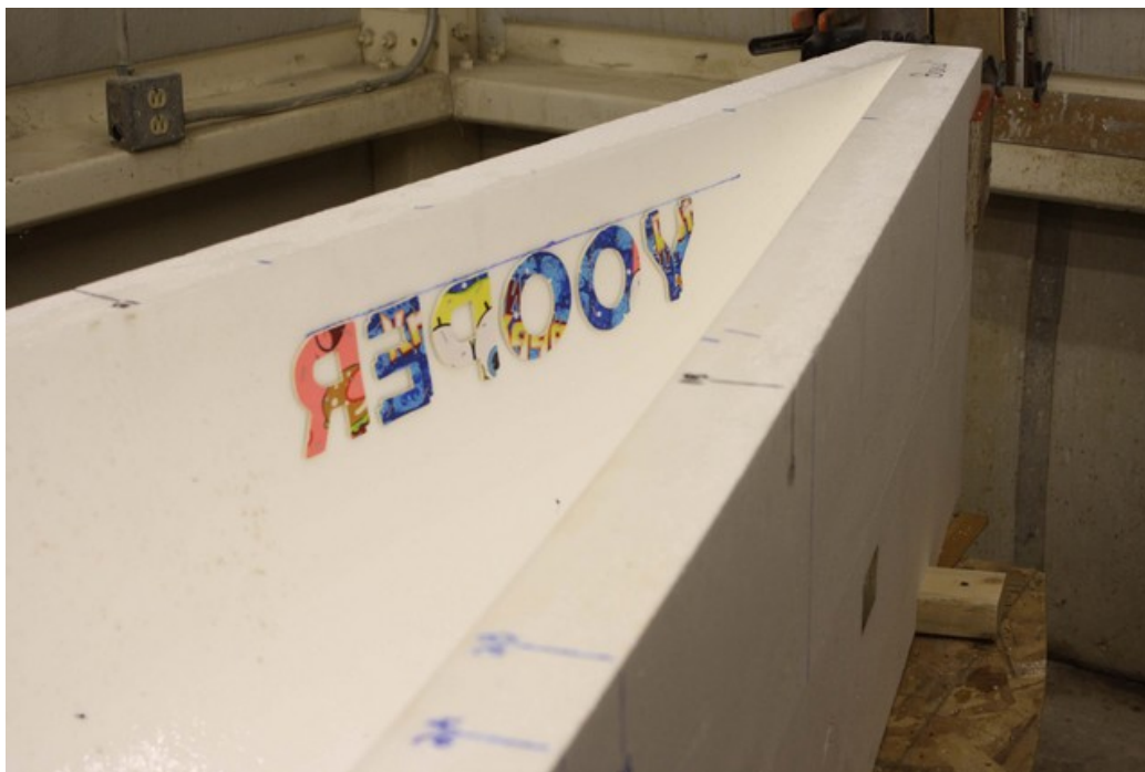
Exterior inlays were cut from vinyl placemats and secured to the mold using staples.
