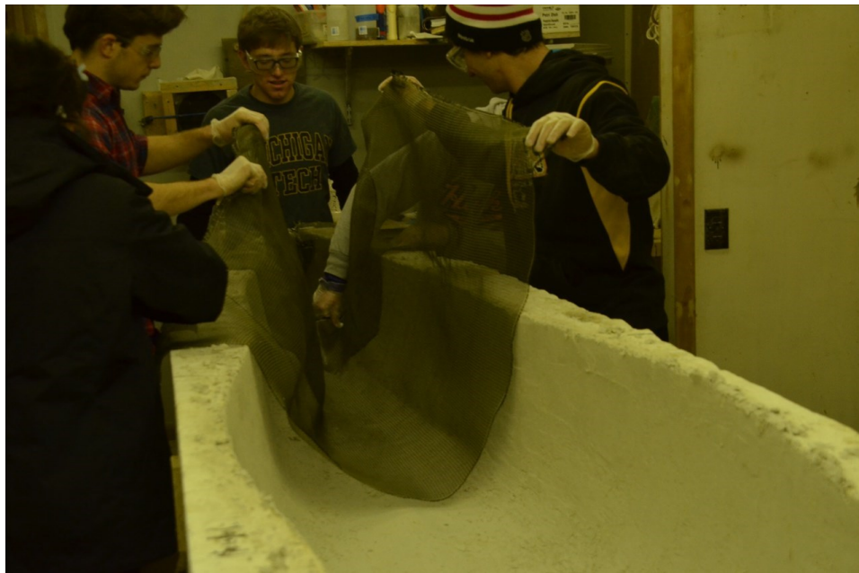
Above, the reinforcement team lays the first layer of Kevlar reinforcement. The transverse orientation of the first layer was from gunwale to gunwale.
