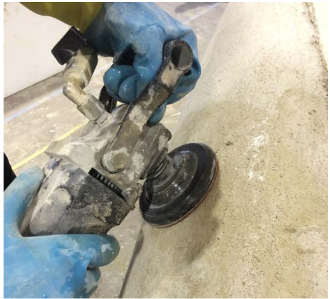
Figure 13: Honing of the canoe
