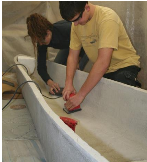
Hand and mechanized sanding was used to smooth the interior and exterior of the canoe.
