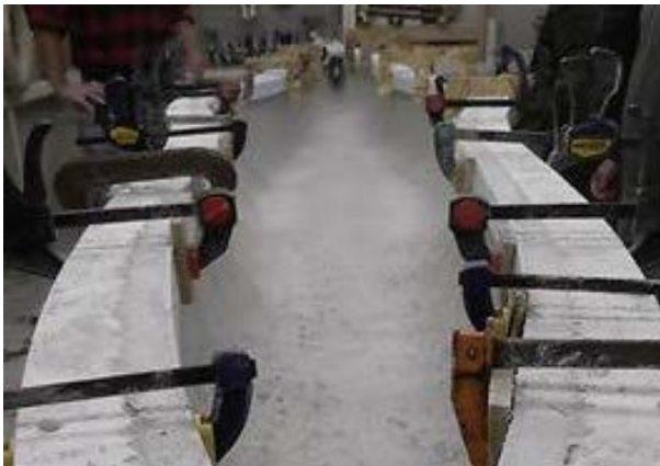
Figure 9: Clamps were used to hold the gunwale caps in place while curing.
