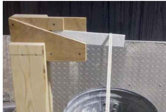
Figure 6: The team designed its own cantilever beam test stand.
