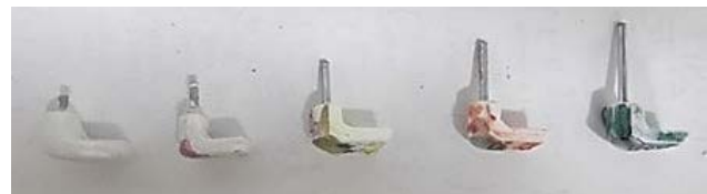
Figure 8: Depth gauges were color-coded for each layer of placed concrete.
