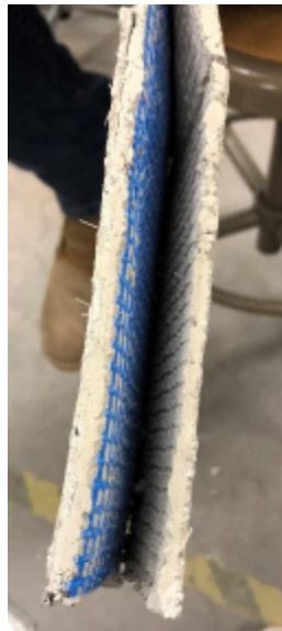
Figure 4: Delamination of a bend test beam containing Panzer 15 reinforcement.
