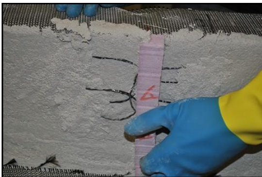
Figure 5: Loose-strand reinforcement being integrated into the ribs.
