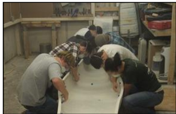
Figure 6: Manually sanding the interior of GENOA.
