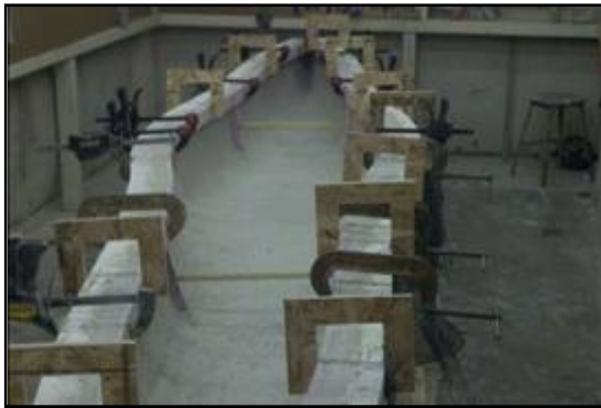
Figure 4: Clamps holding the gunwale caps in place.
