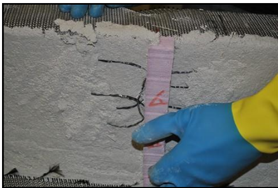
Figure 5: Loose-strand reinforcement being integrated into the ribs.
