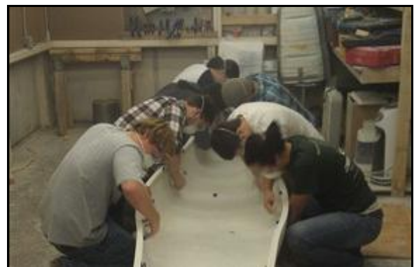
Figure 6: Manually sanding the interior of GENOA.
