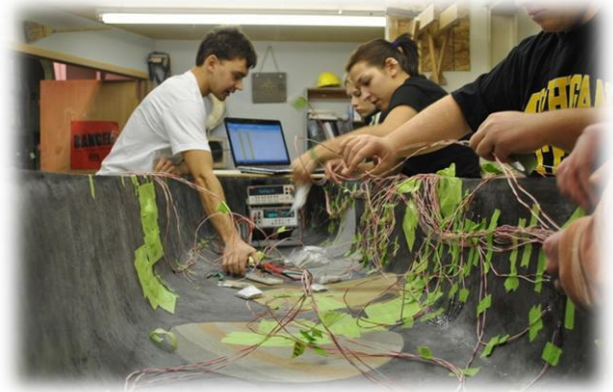
Figure 3: Testing circuits for each of the 73 strain gages on POLARIS .
