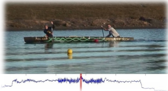
Figure 1: Time-correlated video and testing data helped depict that posting created the highest gunwale stress.
