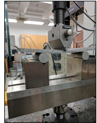
Figure 4. ASTM D790 3-point flexural testing
