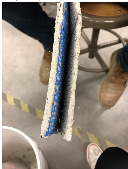
Figure 5: Beam Delamination Testing Results
