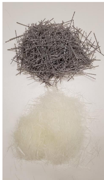
Figure 3: Backfill Fiber Blend. Enduro Prime (Top), PVA RFS400 (Bottom)
