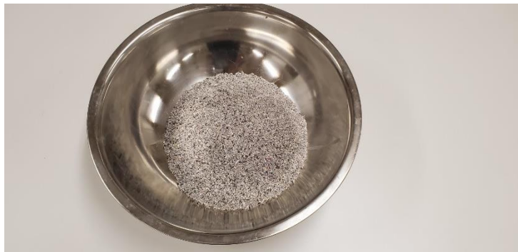
Figure 4: Recycled Concrete Aggregate - Passing #8 Sieve, Retained in #16
