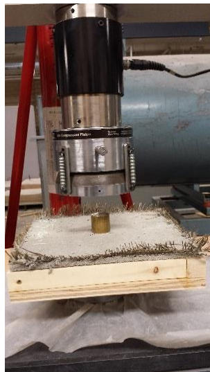
Figure 10: Composite Puncture Testing
