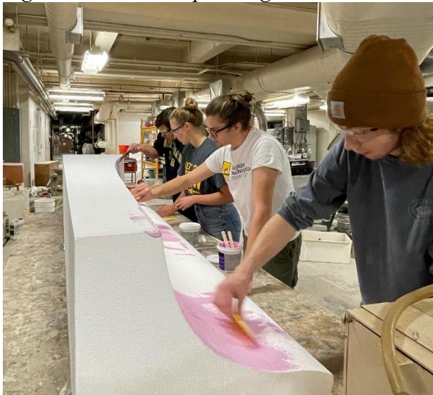
Figure 8: Members Spackling the Mold
