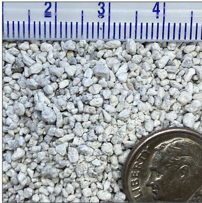
Left: HP Grade number 7. Right: Grade used for as an aggressive filtration media (replacing or supplementing sand, zeolite, or diatomaceous earth) in commercial and residential pool filtration systems.
