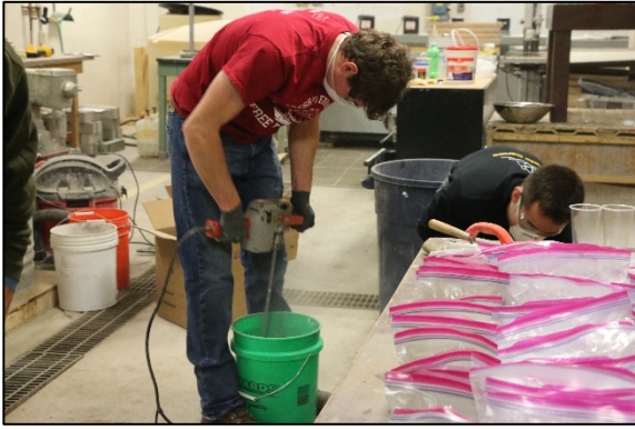
Figure 10. Mixing of Concrete Batch on Casting Day
