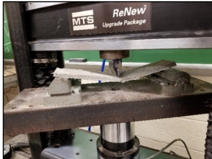
Figure 9. ASTM C1341-13 Flexural Bend Test
